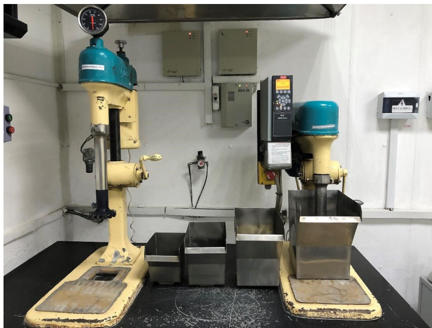
Figure 1. Metso laboratory flotation machines: 3 litre and 0.5 litre cells
