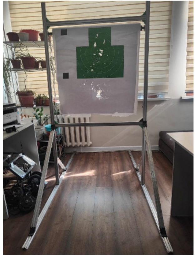
Figure 6. Assembled hardware prototype of the ShootVision stand with a mounted paper target
