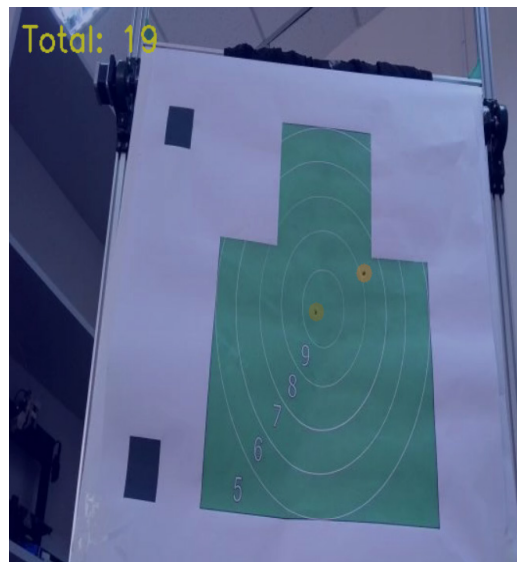
Figure 8 – Example of bullet-hole identification and real-time score calculation.
