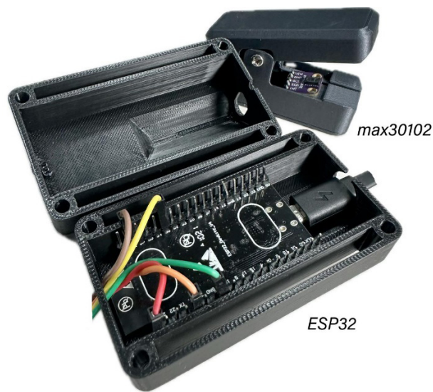
Figure 2 – MAX30102 GY PPG sensor – IoT Device Zhurek.
